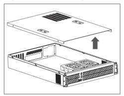
Remove the screws from each side of the Chassis (two on each side). Once the screws are removed, push the top cover to remove from the chassis.
