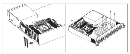
6. Remove brackets and install the Graphics Card, then install the HDD cages.
